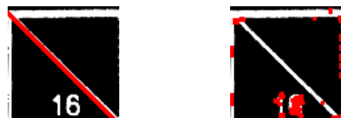
(a) Diagonal line detection (b) Harris corner detection
